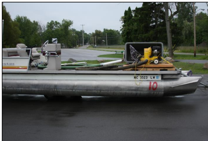
Figure 35. A DASH boat for hand-removal of watermilfoil or other nuisance vegetation.
