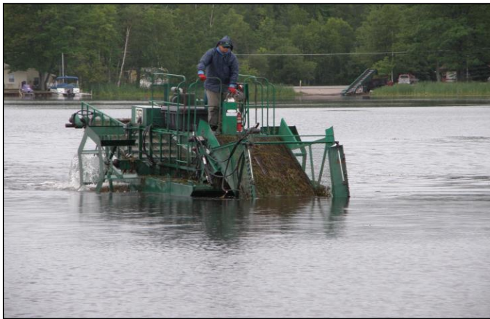
Figure 34. A mechanical harvester. Photo courtesy of Dave Foley.
